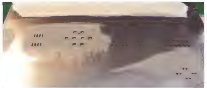
Figure 13. Solder paste spread across the stencil.
